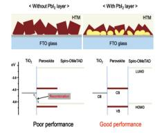
The influence of the unreacted  $Pbl_2$  to the performance of perovskite solar cells is investigated. The optimized morphology of the  $Pbl_2$  under layer is found to be essential to form a dense perovskite layer preventing recombination by direct contact between  $TiO_2$  and a hole transporting layer, and increase the charge collection efficiency.
